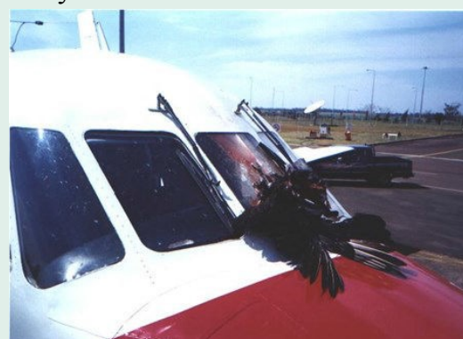
Figure 1. Damage resulting from wildlife strike
